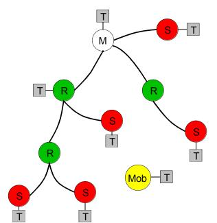
The figure left illustrates a possible structure of a radio modern network.
