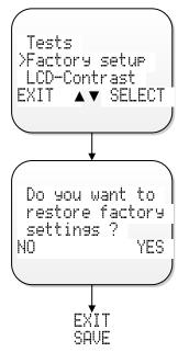
Enter the settings menu first by pressing SETUP button (■) on the top level view.
